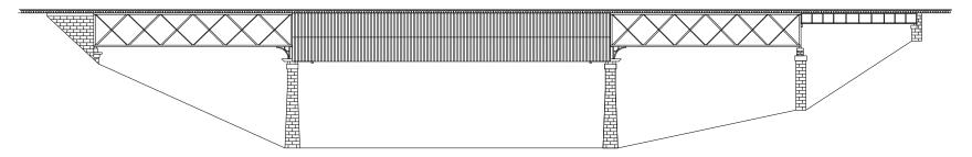
The side spans were replaced by the D&H c.1892 and the center span was covered with wood siding.
