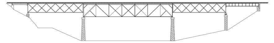
The side spans were replaced by the D&H c.1892 and the center span by 1905 with a pin connected truss. There is no evidence of when the southern span was added so I am doing it here.
